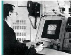
Human Computer Interaction Creator Ivan Sutherland using Sketchpad around 1963 – the origin of computational design.
