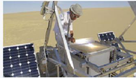
Markus Kayser, Solar Sinter, 2011 This solar-powered 3-D fabrication device is guided by digital modelling software to transform sand into glass sculptures.
