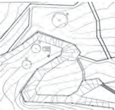
7.17 Plan of main path showing expansion joint positions. 'As built' plan
